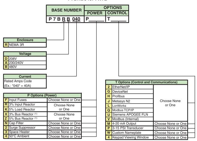
(1) 3% and 5% Bus Reactors are only available as an option on base numbers up to and including P7BR\_D074, A068 and B040; larger drives have a Bus Reactor as standard.
