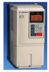
For industrial applications such as centrifugal fans and pumps, the P7 drive is an ideal choice. The drive is provided in Normal Duty ratings with 110% overload capability. V/f control mode, network communication options, and an array of input/output options are available.
