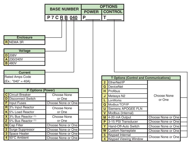
(1) 3% and 5% Bus Reactors are only available as an option on base numbers up to and including P7CR\_D074, A068 and B040; larger drives have a Bus Reactor as standard.
