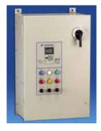
The P7/Bypass package is a 3-contactor style bypass, allowing motor operation from either the drive or across the line. This facilitates drive maintenance while the motor continues to operate. The P7 and P7/Bypass have been designed for flexibility in providing the features and options commonly demanded by facility designers.
