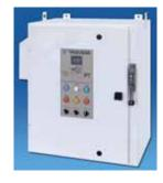
The P7/Bypass package in a NEMA 3R enclosure is a 3-contactor style bypass, allowing motor operation from either the drive or across the line. This facilitates drive maintenance while the motor continues to operate. The P7 and P7/Bypass have been designed for flexibility in providing the features and options commonly demanded by facility designers.
